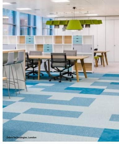
considerably to total sound absorption. The use of Flotex and Forbo carpet tiles reduced walking noise in a neighbouring room by up to two classes (10 dB). Resilient floors scored less impressive results of course, though Marmoleum was more effective than wood and stone, for example.
